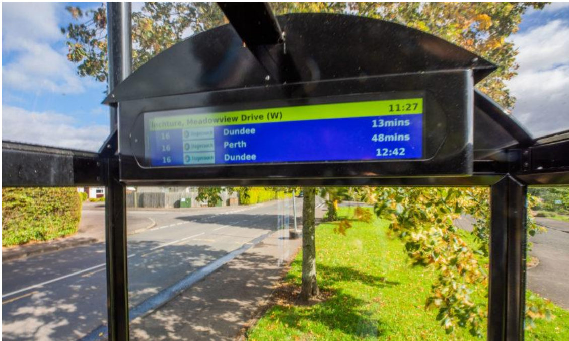
Figure 2.12: Electronic real-time information screens at a bus stop in Scotland showing estimated arrivals for all services 32
