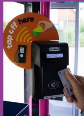
Figure 2: On board payment system in Leicester (Source: Ticketer)
